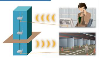
By deploying access points along the IP network, the IP advanced radio system can communicate all the way from the basement to the top floor. The IP110H can access the nearest access point and can roam between access points\*. \*Same SSIDs are required for roaming use.
